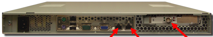
WAN LAN ASI Input (Either can be Used for IP Input or Output)
